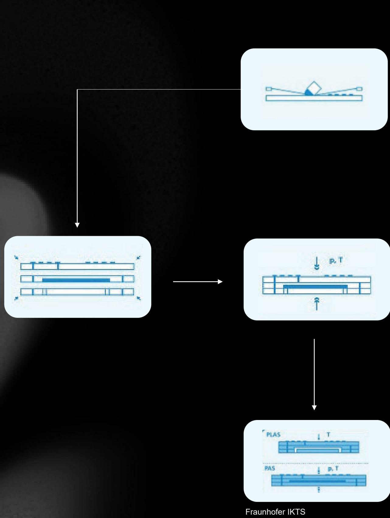
Holes are punched in the green tape, which are then filled with a metal paste. After drying, the conductors, resistors, capacitive and inductive layers of sensory structures are printed by screen printing.
